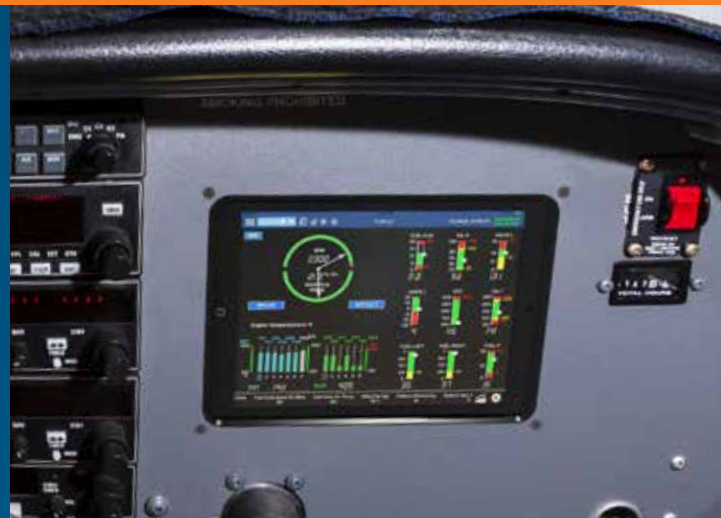
iPad Mini with iFDR Pilot Pro App Displaying Engine Data
